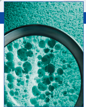
Breathable, moisture regulating cell structure, similar to that of natural sponge.
