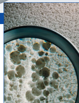
Breathable and moisture regulating cell structure, similar to that of a natural sponge.
